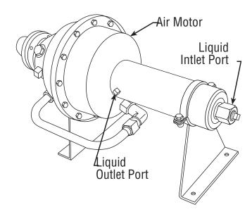
These Sprague Products hydraulic pumps move relatively large flows of liquids at low to moderate pressures. The pumps deliver liquid with each up and down stroke of the liquid piston rather than, like other pumps, pump only with a down stroke. The pump's air-driving action is the same as the Sprague Products air driven S-216-J series hydraulic pumps Being air driven, these double-acting pumps are non-arcing and non-sparking, safe for use in hazardous or confined areas.
